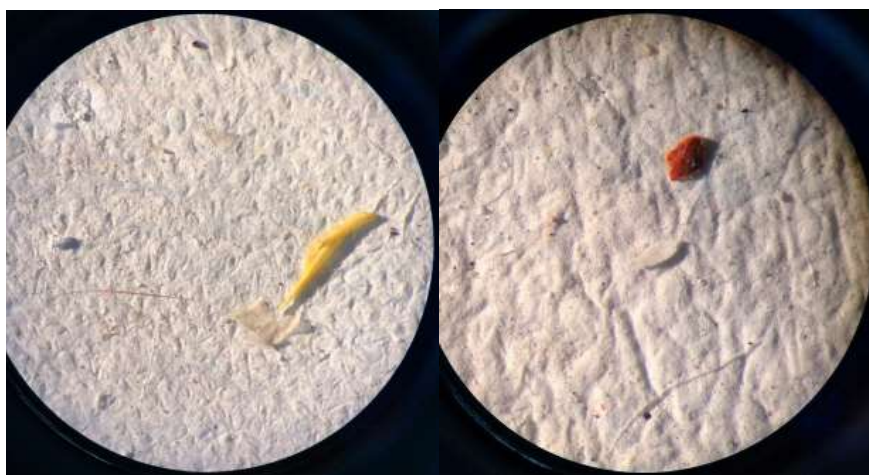
Figure 2. Images illustrating the diversity of size and types of microplastics in biosolids following wet peroxide digestion with 50% H 2 O 2 . Left filter – 16 x magnification; right filter – 32 x magnification.
